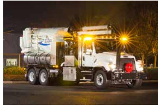
methods. It prevents accidents and injuries for field operators and the public. Hydro excavating is quicker than traditional methods of excavation, allowing field crews to perform repairs with less outage time for customers.
