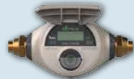
The second type of water meter has an electronic or digital register with a series of numbers much like an odometer in your car. With all water off, look at the numbers on the far right. If the numbers continue to turn, it is an indication of a leak.
